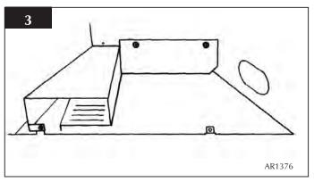
Then remove the two knockout holes on the rear of the box using a sharp hammer blow, Diagram 4.
